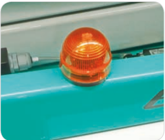
Flashing beacon warning for machine in action.
