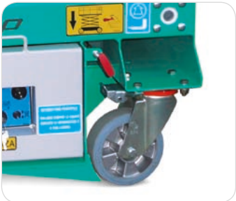
Swivel caster interlock for straight line driving.
